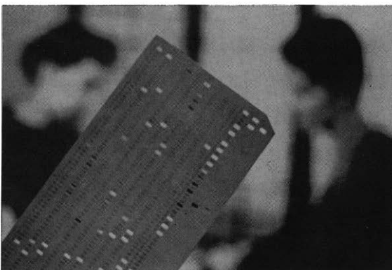
DATA CARDS are fed into the IBM sorter, and only the ones which meet the new client's requirements are retained.
